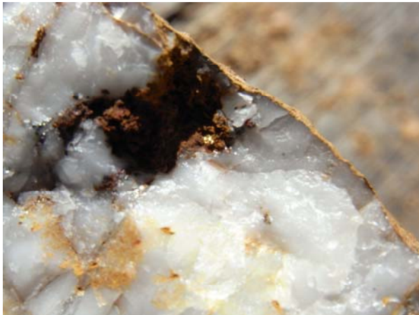
Plate 1: Visible gold grain in quartz vein (Sample QV332904) from workings associated with the Saint Patrick workings in the Mesothermal Reefs area (Palmtrees Project) 5km south of Clermont. Rock Chip assays for the sample yielded a result of 51.4 g/t Au.
