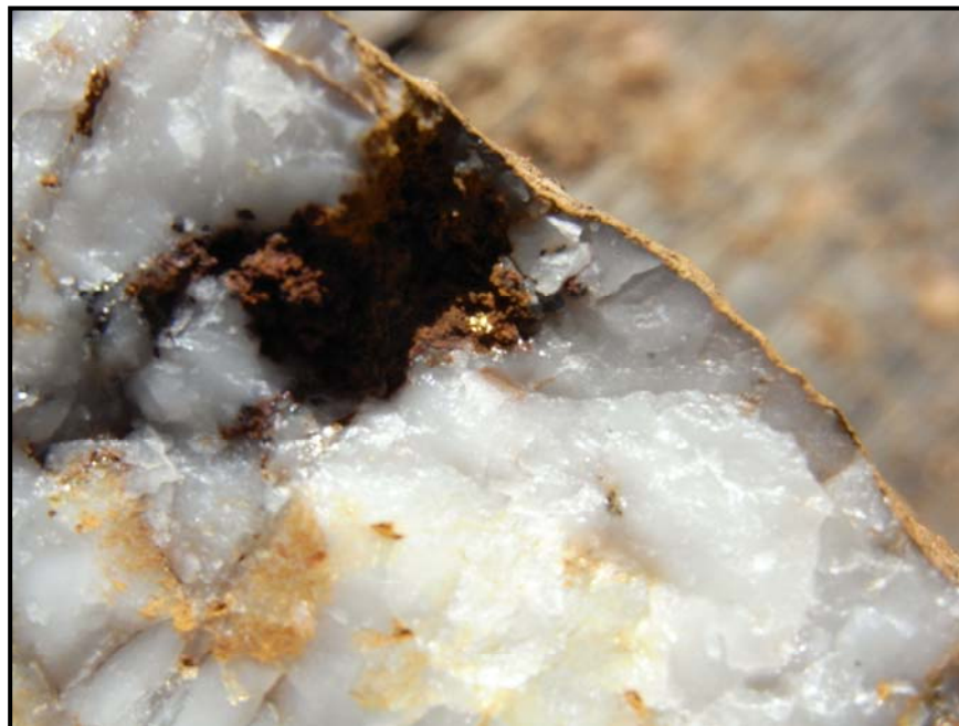
Figure 2: Visible gold grain in quartz vein (Sample QV32904) from workings associated with the Saint Patrick workings in the Mesothermal Reefs area 5km south of Clermont. Rock Chip assays for the sample yielded a result of 51.4 g/t Au.
